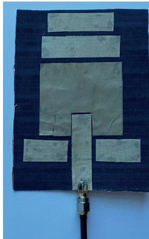
Figure 2 and 3 below shows the fabricated design of the textile Yagi-Uda antenna with a jeans substrate. The Nano VNA analyzer is used to indicate the return loss of the antenna.
