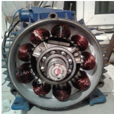
Figure 3 Photo – Symmetrically wound 9 stator windings
